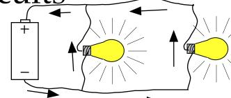
1. Compare the brightness of the lights in the PARALLEL circuit to the series circuit.
